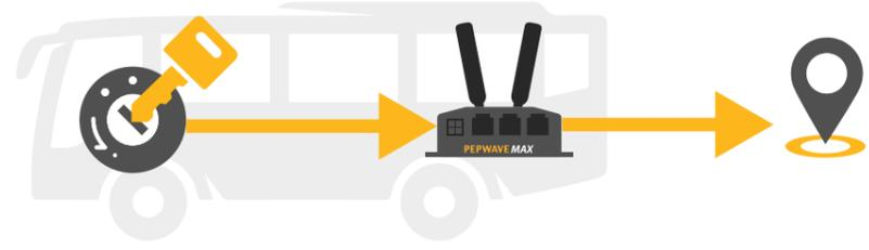
The MAX Transit Mini has specialized features for vehicular deployments. Ignition sensing, which detects the ignition status of the vehicle, enables the device to turn on and off as the vehicle starts up and shuts down. It is also equipped with GPS, enabling you to track its movements. With InControl's fleet management, you can review the route history of all your vehicles from any web browser.
