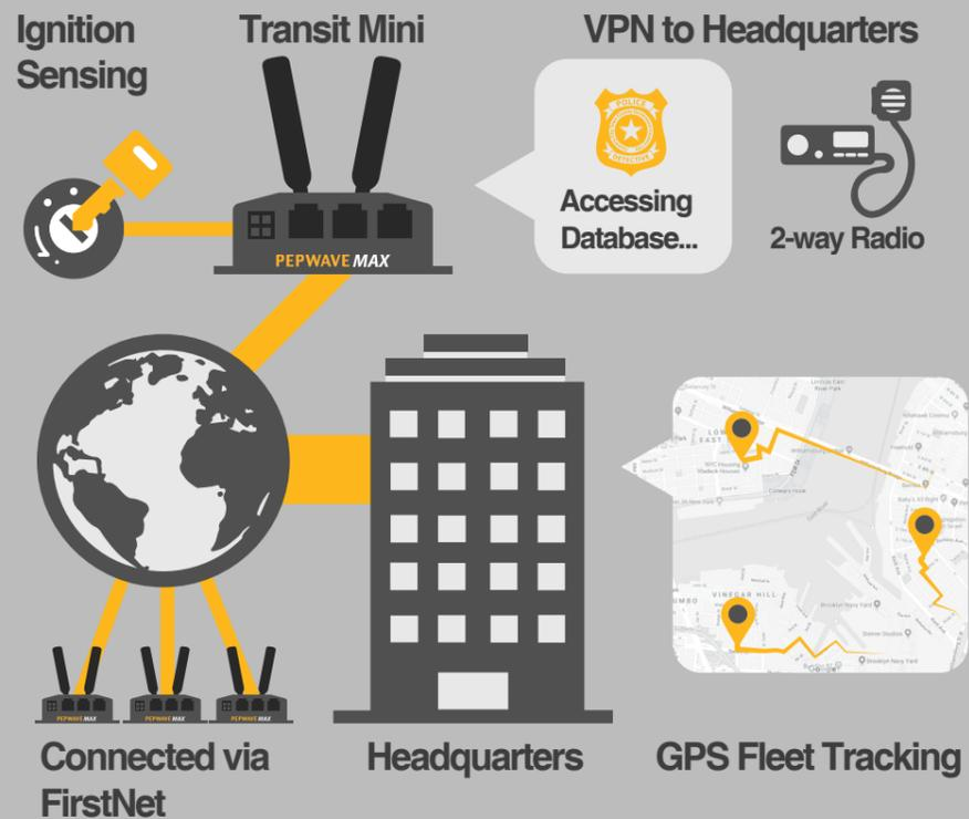
Using the MAX Transit Mini, officers on the field can connect to headquarters using FirstNet. Using the redundant SIM slot, the device can failover to commercial LTE as needed. By building a PepVPN to headquarters, 2-way radios such as TETRA, NXDN, and DMR can be used between multiple remote sites, enabling the entire force to seamlessly communicate as if they were connected to the same repeater. Finally, the Transit Mini can broadcast a mobile hotspot, connecting cameras and other equipment.
