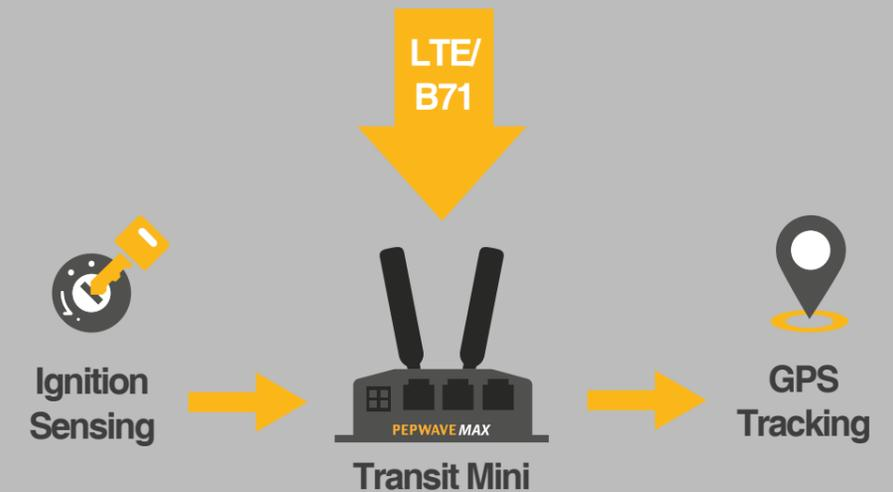
The MAX Transit Mini provides cellular connectivity for passengers. It connects using LTE, supporting band 71 for improved range and signal penetration. This means the Transit Mini will stay connected even in remote areas where other bands drop off.
