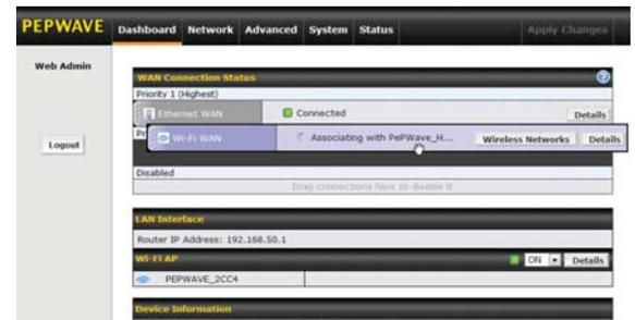
Arrange connection preference easily with MAX's easy to use drag and drop interface, the MAX will automatically switch to the best connection available.
